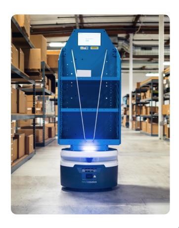
At this stage, use of robots in a temperature-controlled environment is conceptual, but theoretically possible as they are able to withstand temperatures as low as -25°C. Their only constraint is they are not immune to condensation—which means they are limited to staying within a single temperature zone. However, if robots remain isolated to a freezer or chilled zone, this shouldn't cause a problem.
